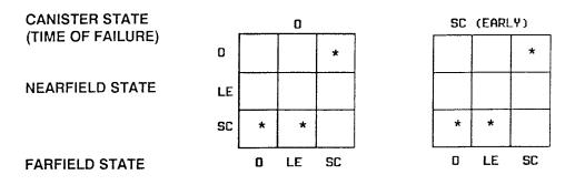
Figure 4-4. Formulation of scenarios by combining different barrier states. (\*) denotes an improbable combination.
